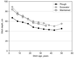
Figure 1. Average depth of original ditches made by plough or excavator, and maintained ditches made by excavator as a function of ditch age
