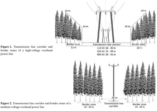
Figure 2. Transmission line corridor and border zones of a medium-voltage overhead power line
