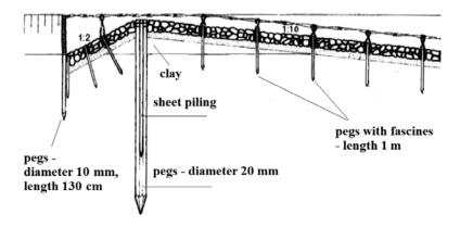
Figure 1. The design of the weir
