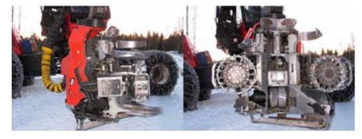
of feed rollers was three, the maximum feeding speed was 5 m/s and cutting was performed with a chainsaw (Komatsu Forest AB).
