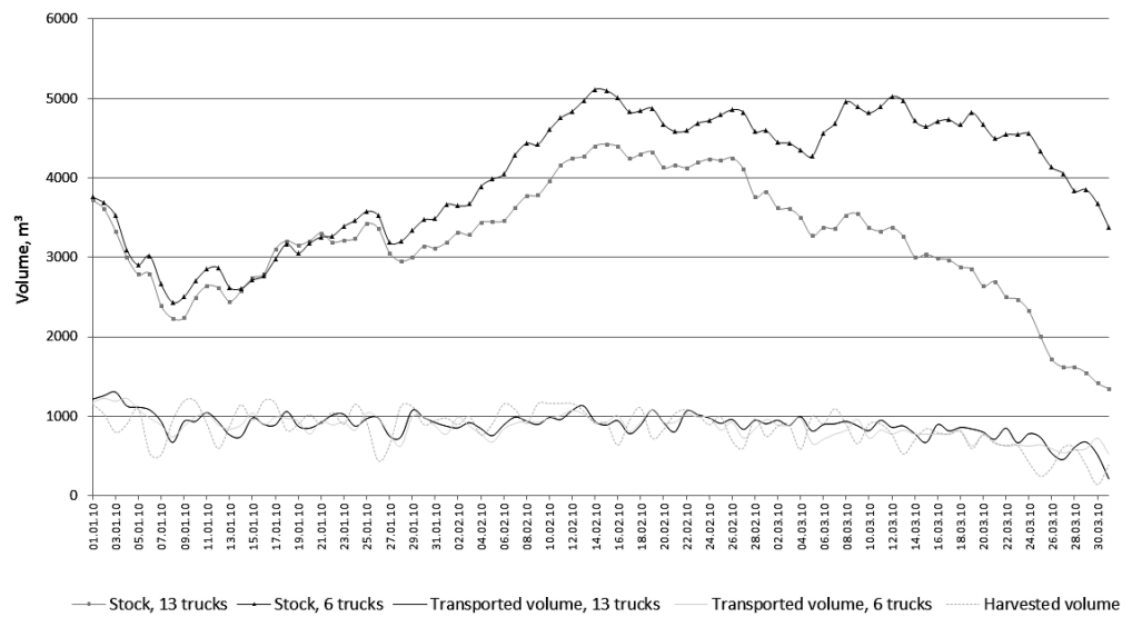
Figure 7. Results of from Case study 2 for the existing fleet (Basic, 13 trucks) and reduced fleet (Advanced, 6 trucks). The figure shows the daily harvested volumes, transported volumes, and the development of the roadside stocks (m 3 ) for both the existing and reduced fleet over the three-month period.
