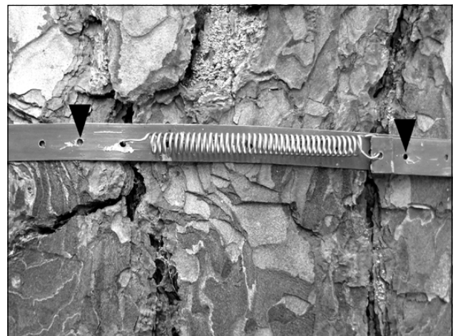
Figure 2. Band dendrometer installed on pine tree; arrows show measuring points for the circumference growth
