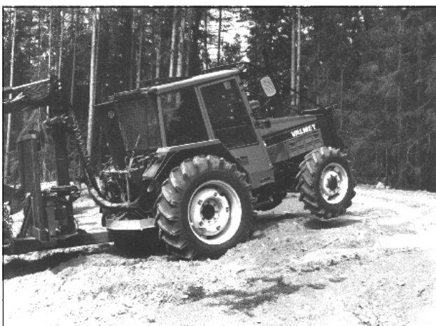
Figure 4. Rearing tractor during uphill trial with heavy load on the hitch hook, four wheel-drive but no cylinder force. (It was possible to continue up the hill after engaging the cylinder force)
