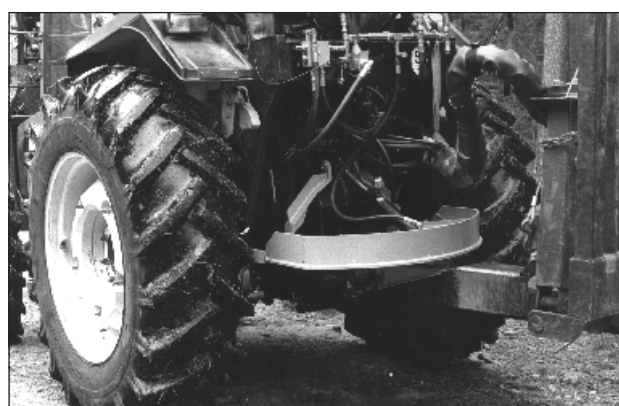
Figure 1. Design of the hitch hook device
